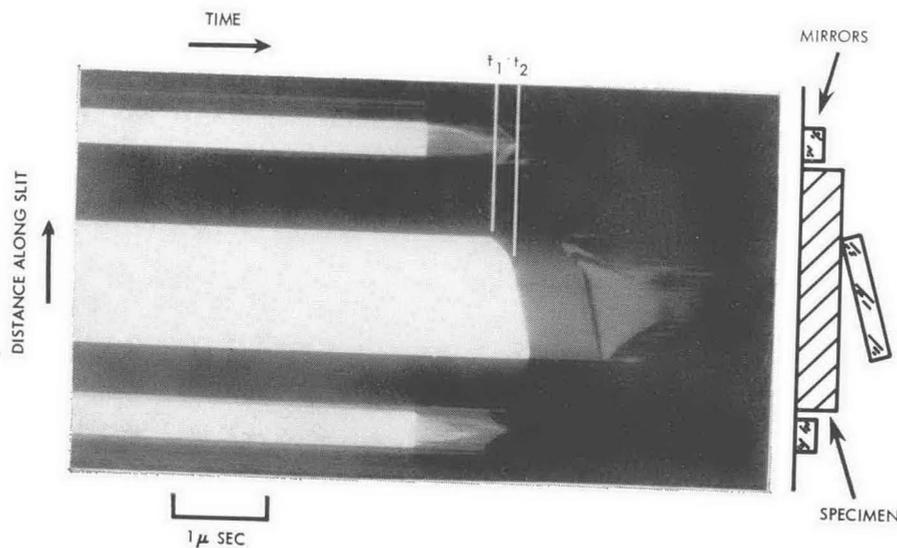
Fig. 9. Streak camera photograph of two shocks in  $\text{BaTiO}_3$  (arrival times  $T_1$  and  $T_2$ ) affords both shock and free-surface velocities by measurement of the slope of successive light traces.
